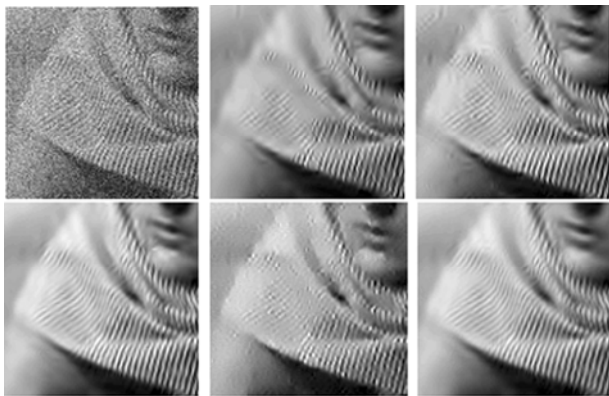
图3 \sigma = 30 时 Barbara 有噪图像的降噪。从左到右、从上到下分别为: 有噪的图像, PSNR = 18.59dB; FeatShrink, PSNR = 25.90dB; ProbShrink, PSNR = 27.14dB; BiShrink, PSNR = 27.61dB; SURE-LET, PSNR = 26.01dB; 本文方法, PSNR = 27.78dB。
